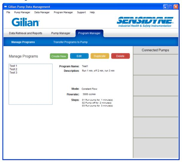
Creating programs is simple and easy on the PC using the Data Management system, making it convenient to edit and manage a library of sampling programs. The program capabilities of the GilAir Plus are described in detail in the GilAir Plus Operators Manual. Please refer to that document for a comprehensive specification and examples. The presentation here covers editing, saving, loading and managing programs in the PC application.
