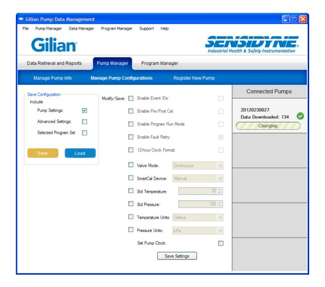
This screen provides the ability to control advanced settings and allows saving the current configuration of the pump to a profile for reuse. It also facilitates loading of previous configurations and the application to a selected pump. This screen is only available when a pump is docked.
