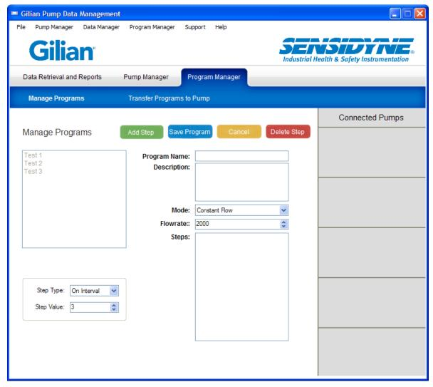
Programs must specify the control mode desired, Constant Flow, Constant Pressure High Flow or Constant Pressure Low Flow and the set point at which to operate. Please note that programs using Constant Pressure modes are always specified in pressure units of inches of water.
