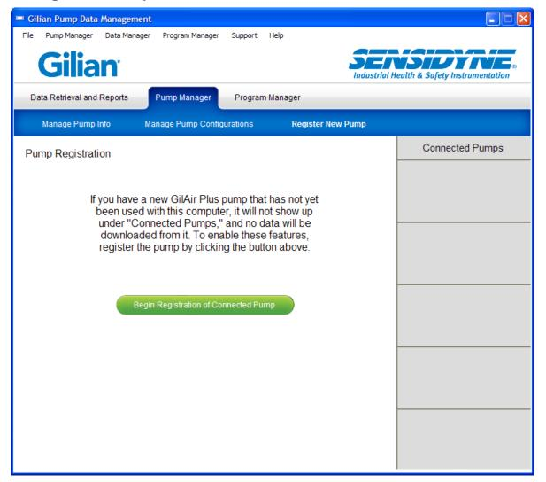
Registering a pump with your PC is required before communication is possible, and before sampling logs can be downloaded. A pump can be registered on any number of PCs. The Register New Pump screen is not available while any registered pumps are mounted on the docking station.
