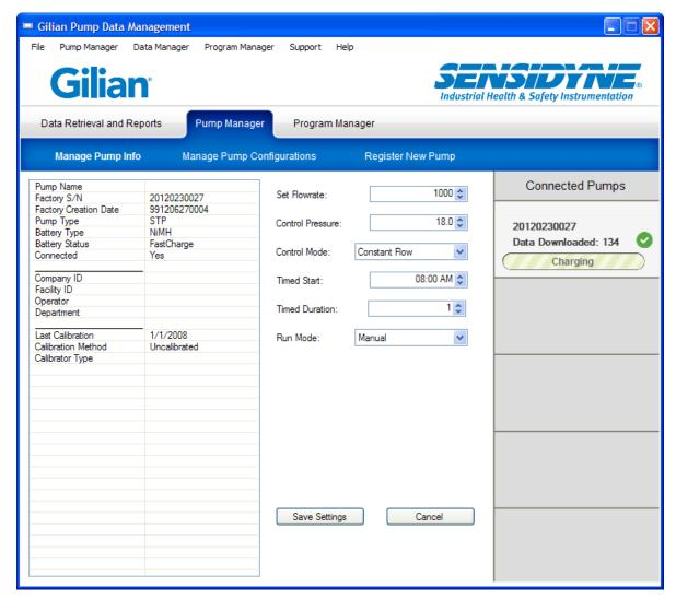
The Manage Pump Info screen displays two main columns of information, (1) a table listing information about the selected pump including the serial number and pump type, and (2) a set of six basic settings that can be changed in the pump. Changes to the fields contained on this screen will be lost if a different pump is selected before saving the values or if the pump is removed from the Dock. Manage pump info is only available while a pump is connected.
